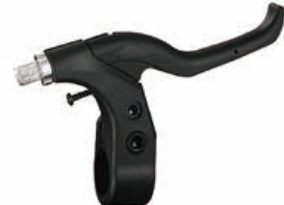
XW-BL-06 2-3fingers nylon-compsite lever& bracket with steel insertion and return spring
