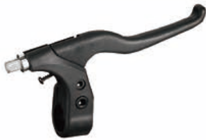
XW-BL-04 4fingers nylon-compsite lever& bracket with steel insertion and return spring
